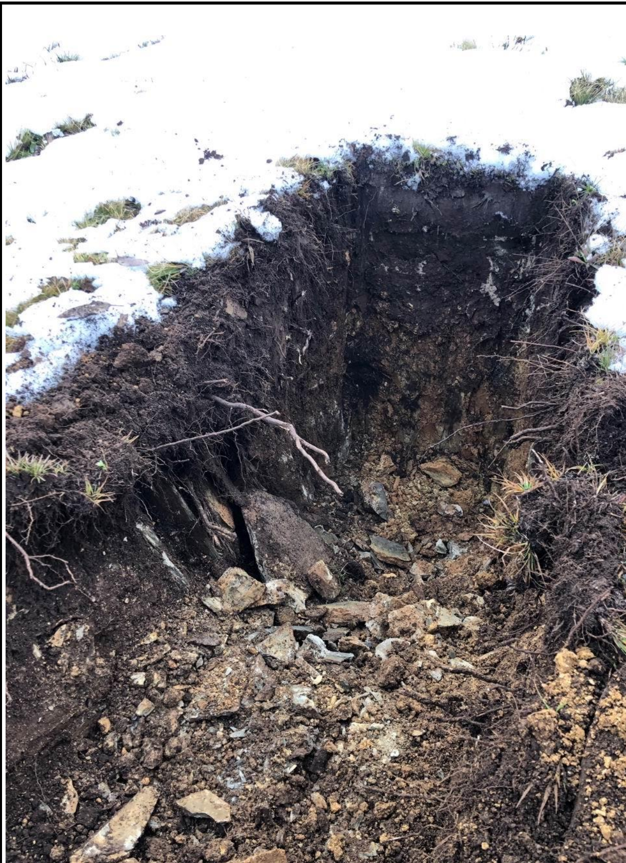
Photo 10 – 10/7/2020 – View of the subsurface profile of test pit 3T, showing topsoil, directly underlain by medium strong slate bedrock.
